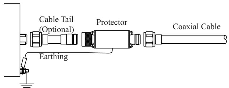
Figure 3: Connection of Novaris Coaxial CCTV Protec-
