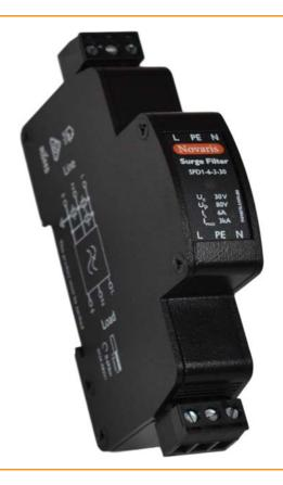
The Novaris SFD2 range of surge filters is designed for protecting floating AC or DC power supplies. Applications include DC power supplies, balanced circuits for rail applications and single phase IT systems.
