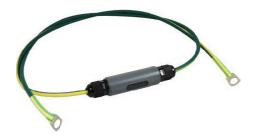
**Novaris EC Earth Clamps** provide a means to electrically clamp different earthing systems during transient disturbances. Applications include computer rooms and in the bonding of cable sheaths to ground where direct bonding would introduce interference and "earth loops".
