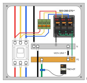
Figure 6. Surge Diverter - Main Switchboard.
