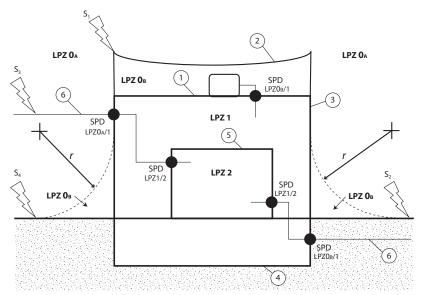
Figure 3. Lightning Protection Zones.
